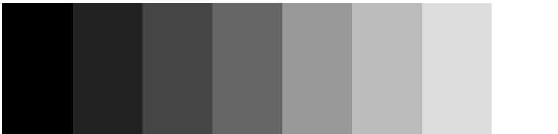
Figure 11-13 Mono Bar Test Pattern
